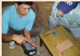
Image Ref. 3.13 Measurement of a single brick Source: Junji Kiyono
