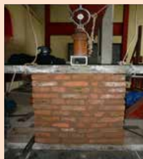
Image Ref. 3.16 Material strength was also estimated by static loading test. Shear loading test Source: Junji Kiyono
