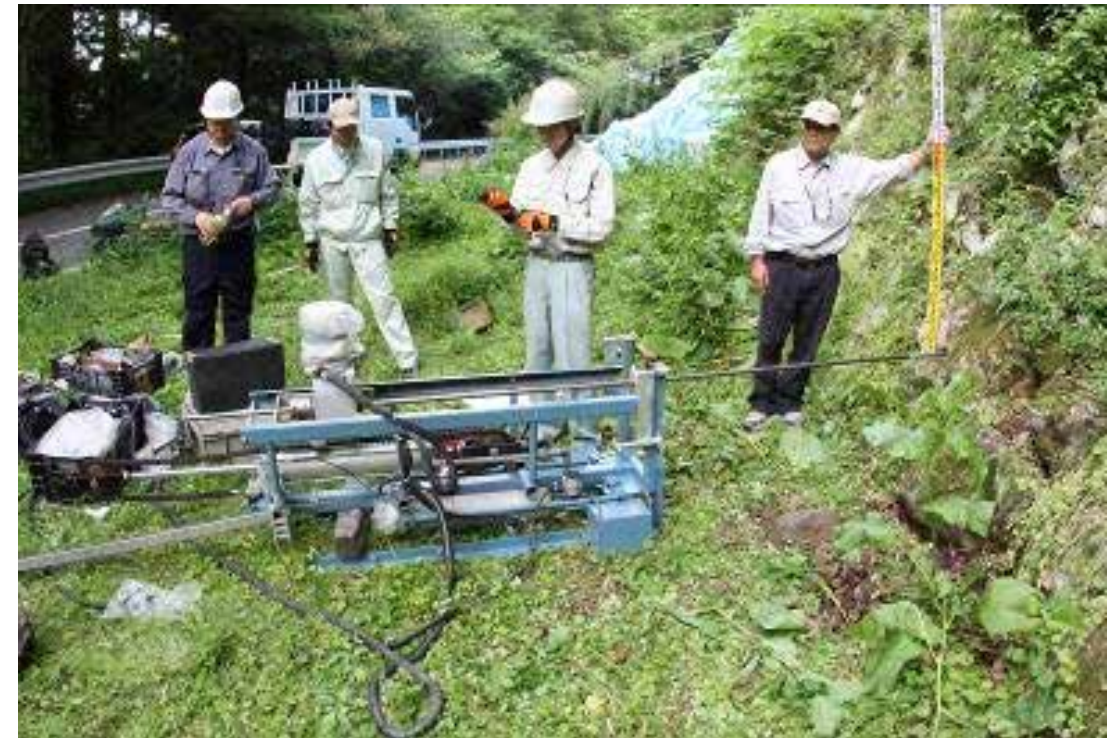
▲ Image Ref. 3.35 INSWS, new in-situ testing device, used in Sendai-ryo-castle Source: Ryoichi Fukagawa
