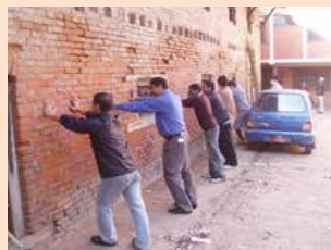
Image Ref. 3.18 Free vibration test Source: Junji Kiyono
