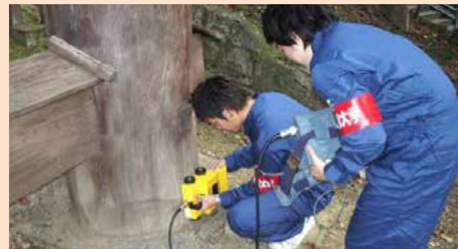
Image Ref. 3.19 Electromagnetic radiation inspection at Kiyomizu-dera Temple Source: Kazuyuki Izuno
