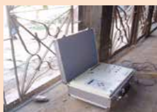
Image Ref. 3.17 Microtremor observation device Source: Junji Kiyono
